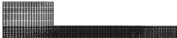
Fig. 10 Computational grid used for the sharp-edged orifice
